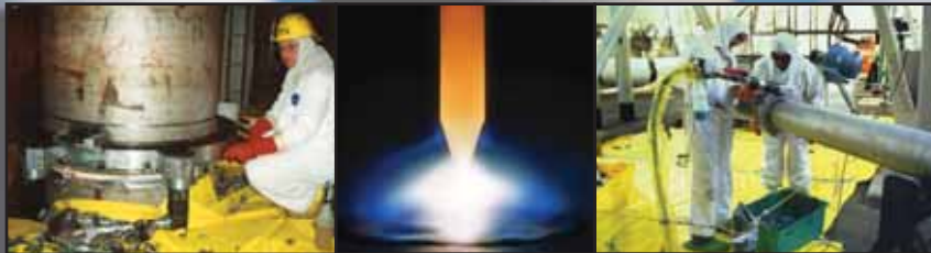
Above: A critical weld in a nuclear power plant being performed by Tri Tool Thermal Services™ with Tri Tool's new DualARC™ dual-process TIG-MIG orbital weld head and OrbitMaster™ Digital Programmable Welding Arc Controller.
