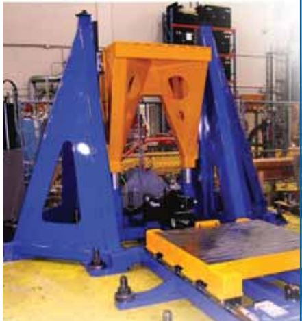
RIM table for seismic testing
